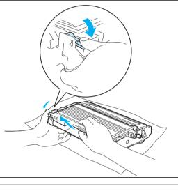
1 Put the drum unit and toner cartridge assembly back in the printer.
