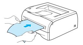
3 Remove the printed even-numbered pages from the output tray and put them back into the manual feed slot in the same order one by one. Place the paper with the side that is going to be printed on (the blank side) face up. Follow the instructions on the computer screen.
