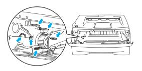
Push down the blue lock lever and take the toner cartridge out of the drum unit.
