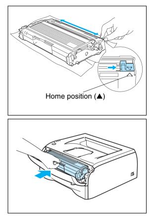
4 Put the drum unit and toner cartridge assembly back in
