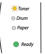
The **Toner** LED alternates turning on for 2 seconds and off for 3 seconds.
