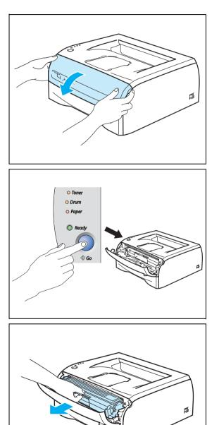
Press and hold down the Go button for about 4 seconds until all the LEDs light up. Once all four LEDs are lit, release the Go button.
