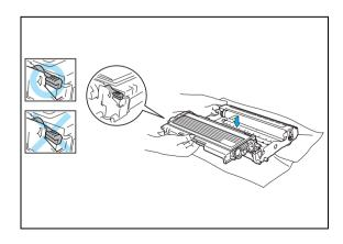
7 Put the drum unit and toner cartridge assembly in the printer.
