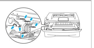
3 Clean the primary corona wire inside the drum unit by gently sliding the blue tab from right to left and left to right several times. Return the tab to the home position (▲) before you put the drum unit back in the printer. If you do not, printed pages may have a vertical stripe.
