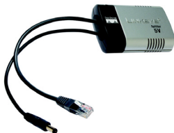
Figure 2: Ethernet OUT and Power Cables
