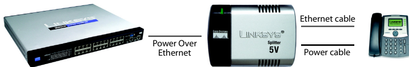
Figure 4: Power Over Ethernet Splitter Used with a Power Over Ethernet Enabled Switch and IP Phone
