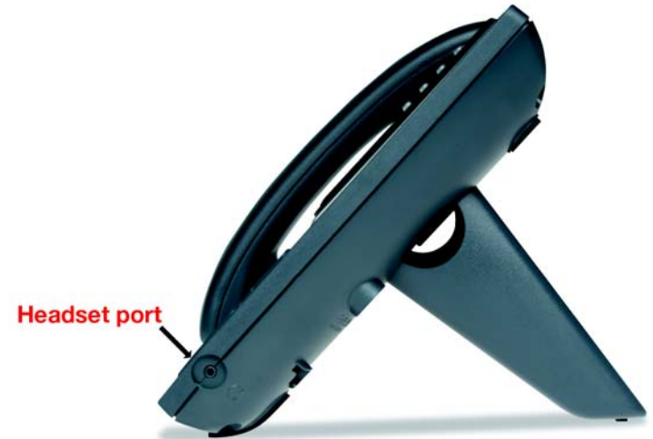
Figure 2-2: desk stand attached to phone (step 5)
