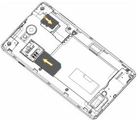
3. Expand the device memory with a microSD(HC) up to 32GB (optional):
