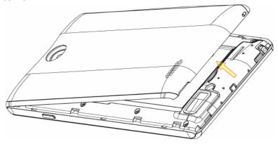
Insert your SIM card carefully into the SIM slot as shown:
