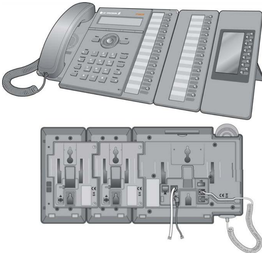
Figure 4.5-4 LIP-8000 DSS Installation (12DSS + 12LSS)
