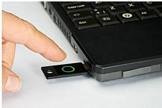
Under the green ring or dot, is a solid-state capacitive touch sensor that reacts on touch by a finger. There are no moving parts and unlike traditional mechanical or membrane touch buttons, no explicit force is necessary.
