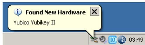
The device is recognized as a Human Interface Device (HID), and the operating system installs the built-in drivers for it
